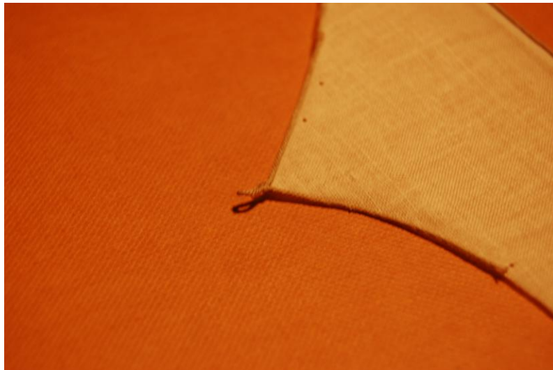
Clews glued to the pattern. Outside edge aligns with outside edge of pattern.
